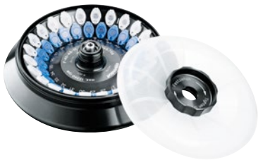
Rotor F-45-48-11 > Max. speed: 18,213 × g (12,700 rpm) > Max. capacity: 48 × 1.5/2.0 mL tubes
