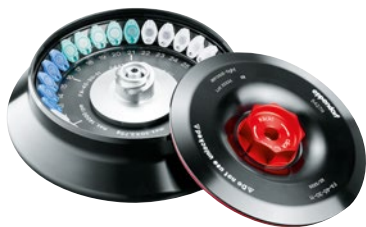
Rotor FA-45-30-11 > Max. speed: 20,817 × g (14,000 rpm) > Max. capacity: 30 × 1.5/2.0 mL tubes > Aerosol-tight with Eppendorf QuickLock® lid
