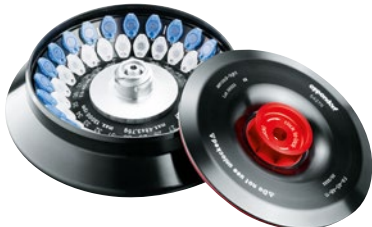
Rotor FA-45-48-11 > Max. speed: 18,213 × g (12,700 rpm) > Max. capacity: 48 × 1.5/2.0 mL tubes > Aerosol-tight with Eppendorf QuickLock® lid
