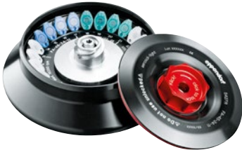
Rotor FA-45-24-11 > Max. speed: 25,001 × g (16,220 rpm) > Max. capacity: 24 × 1.5/2.0 mL tubes > Aerosol-tight with Eppendorf QuickLock® lid
