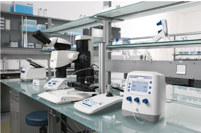
Workstation for microinjection into small organisms
