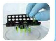
PCR STRIP ROTOR holds two, 0,2 ml 8-strips or 32 x 0,2 ml single tubes
