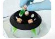
**TUBE ROTOR** holds up to eight microcentrifuge tubes or eight conical or skirted screw cap microtubes
