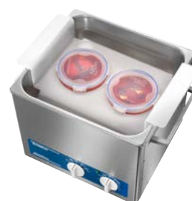
BactoSonic – Ultrasonic bath for gentle removing of biofilms
