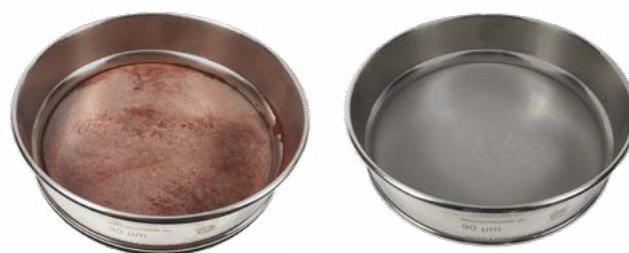
Analysis sieve before and after cleaning
