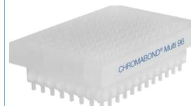
Simultaneous preparation of 96 samples with our CHROMABOND SPE multi 96-well plates are your choice for high-throughput (HTP) solid phase extraction with automated robot systems. Make your SPE more economical by saving time and less consumption of solvent.
