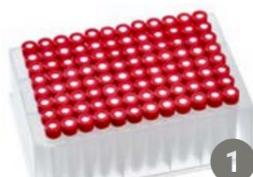
**Deep Well Block, 96 position, PP, filled with 0.35 mL clear-glass micro-insert**
