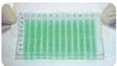
**X-Clear Polyolefin Sealing Film, 96 µm (incl. plastic seal applicator!)**
