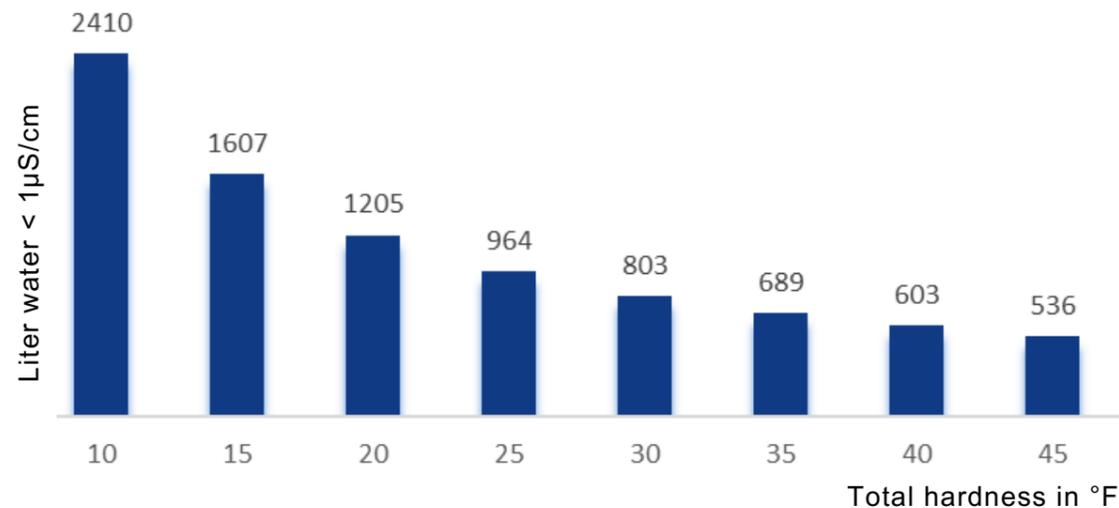
The graph illustrates the volume of water produced below 1 µS/cm with one cartridge. The amount produced depends on the starting hardness of the water. Mentioned values are indicative. Fo
