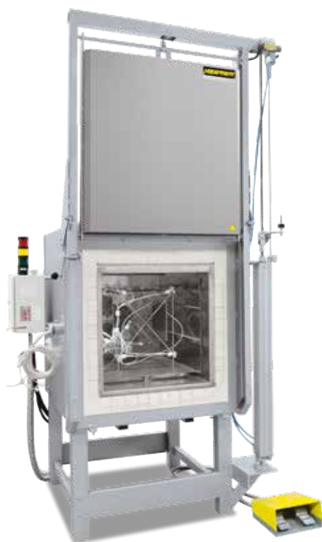
Holding frame for measurement of temperature uniformity
