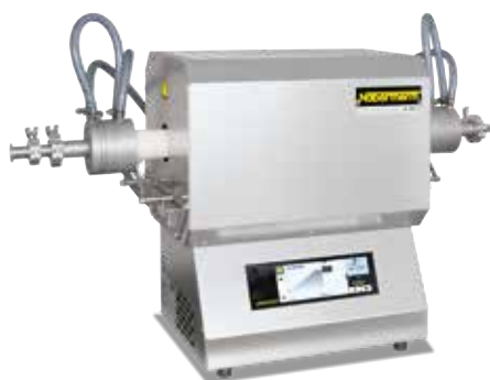
Tube furnace R 50/250/13 with gas supply system 2
