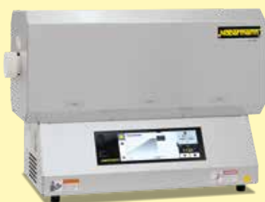
Tube furnace R 50/500/12 with three zone control
