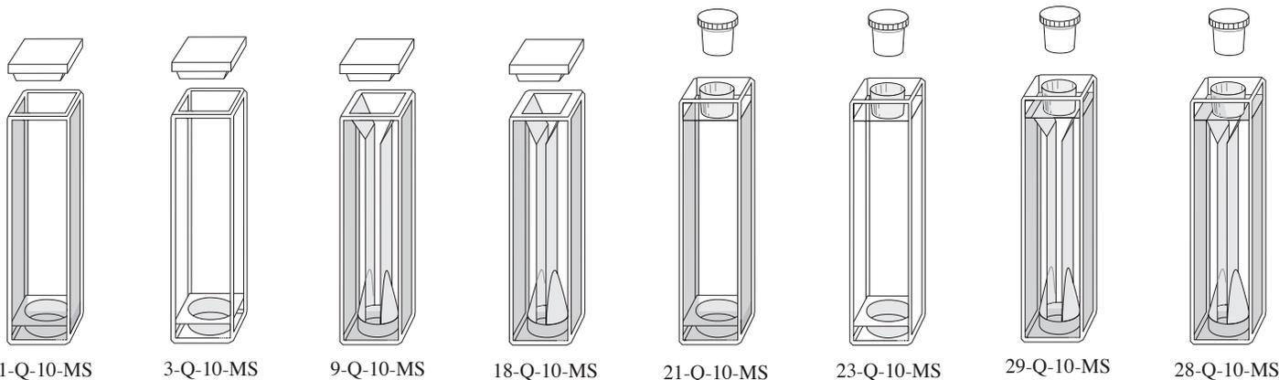
This range of spectrophotometer cells is designed specifically for use with magnetic stir bar type stirrers. The circular recess in the bottom both contains the stir bar and increases the stirring efficiency. Cells are supplied with a PTFE lid or stopper as pictured.
