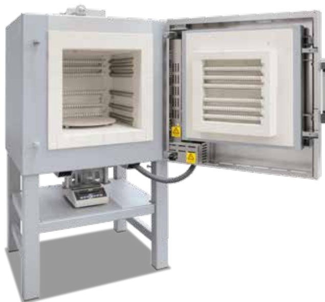
Chamber furnace LH 60/12 SW with scale to measure weight reduction during annealing
