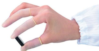
The finger cots made of antistatic natural rubber, with a thickness of min. 0.09 mm, are ideal for applications where the highest precision and fingertip sensation is required. Due to microtexturing, they are also especially handy. Surface resistance: 10E10~120Ω
