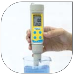
Step 1: Immerse tester sensor in solution
